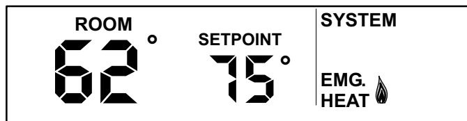
Figure 5. Emergency Heat Mode Enabled
